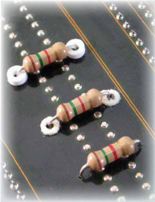
**WASH-AWAYS™** are organic polymer spacers that dissolve in hot water or alcohol. The dissolving spacers locate and reinforce PCB components during soldering operations. After soldering is complete, Wash-Aways dissolve in most aqueous baths and sprays that remove solder flux. This leaves uniform spacing between components and boards to provide free circulation of air, mechanical protection, optimum filleting, and greater accessibility for inspection, cleaning, and conformal coating.
